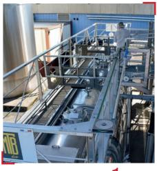
SAFE ACCESS SYSTEM WITH THE MONTE ET BAISSE® FALL PROTECTION SYSTEM
